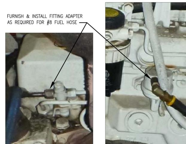
DIESEL FUEL RETURN (DFR) CONNECTION DIESEL FUEL SUPPLY (DFS) CONNECTION
